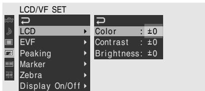
Set color, contrast and brightness of the LCD monitor with the corresponding LCD menu items: Color, Contrast, and Brightness
