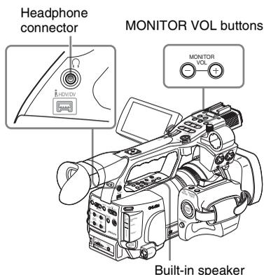
With the headphones connected to the headphone jack, the built-in speaker is turned off.
