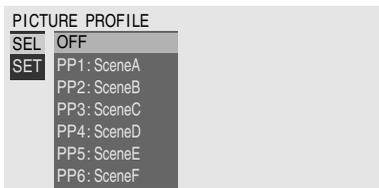
The camcorder is adjusted to the picture quality specified by the selected Profile. (If you select “OFF,” the camcorder will be fixed at the standard picture quality, and no picture adjustment is allowed.)
