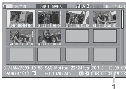
The detailed information of the clip is displayed at the bottom of the screen.
