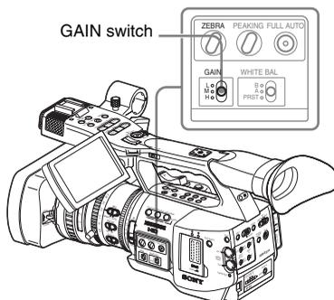
The gain value at each of the switch positions are set at the factory are as follows:
