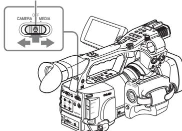
Press the center green button to unlock the power switch and move it from the OFF position to the CAMERA or MEDIA side.
