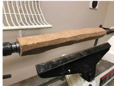
STEP II: CUT OFF EDGES OF BLOCK AND BEGIN TURNING
