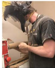
STEP III: TURNING COMPRESSED DOWELS ON LATHE
